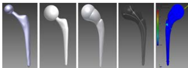
Fig. 4. Design phases of articular spacer
