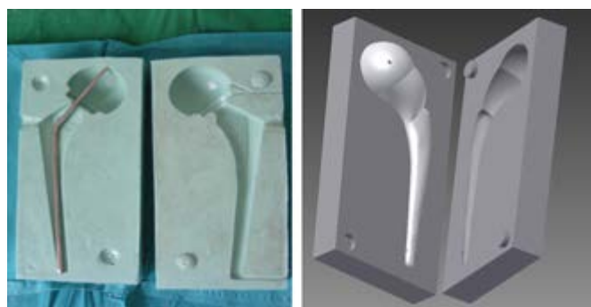
Fig. 5. Virtual and physical mold side by side
