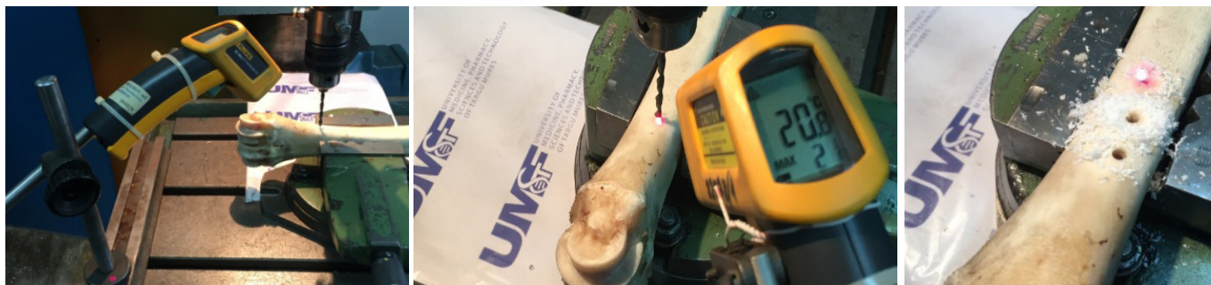
Fig. 1. a. Experimental setup for drilling into bone; b. Temperature measurement in the guide hole during drilling; c. Temperature measurement in the guide hole after drilling
