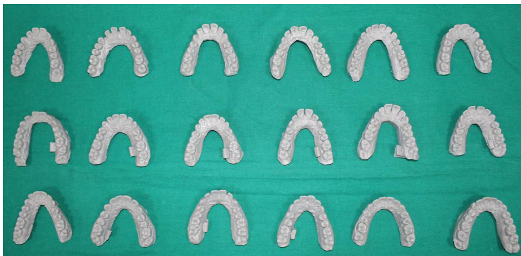
Fig. 1. Reconstructed three dimensionally printed models using Figure 4 Standalone 3D printer based on non-contact membrane Figure4® technology set to their most accurate printing settings.
