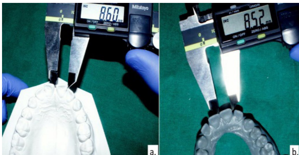
Fig. 2. Manual measurements performed with a digital vernier caliper on - a. Conventional plaster model and b. Reconstructed three-dimensional printed model.
